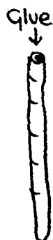
Glue Cotton Brush of goat hair bound with cotton and glued into hole in end of stick
