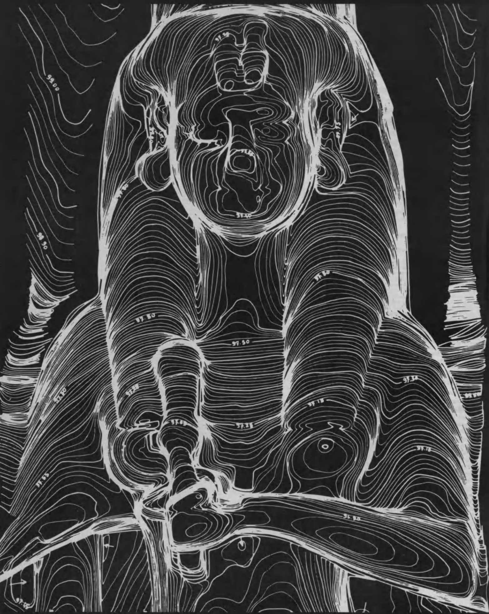
Detail from statue of queen Nefertari is taken from a photogrammetric survey of the façade of the small temple of Abu Simbel.
